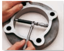
Measuring inside diameter using convenient handle attached to the micrometer.
